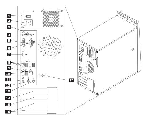
Figure 2. Rear connector locations
